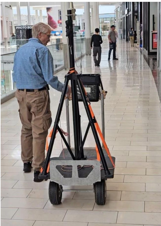
Cart to hold equipment and unity gain antenna above our heads
