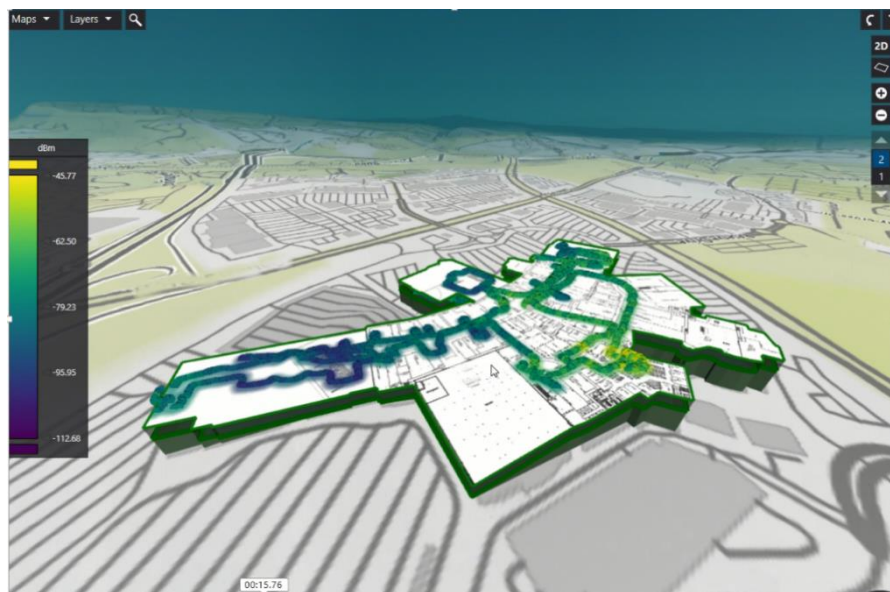
Neon Command 3D display of measurements showing good coverage on the second floor
