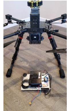
Anritsu MS27100A spectrum analyzer removed from the drone
