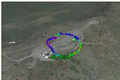
Google Earth display of signal strength measurements taken from the circle flight
