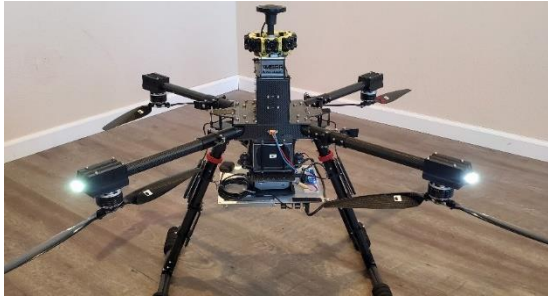
WISPR Range Drone with 7 lb payload capacity
