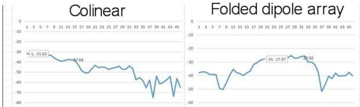
The ANT450 F6 colinear antenna dropped 6 dB at 3 deg downtilt. The ANT 450 D6 folded dipole array maintained signal strength to 3 deg. downtilt.
