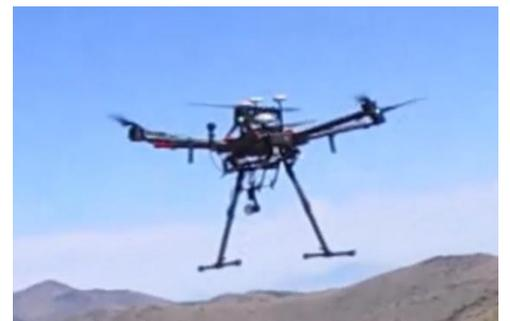
DJI Matrice 600 with spectrum analyzer and vertical antenna
